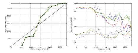
Source (blue) and target (red) magnitude spectra (solid lines), and their corresponding flattened LPC spectra (blue and red dashed lines). Yellow lines are the result of applying the full (yellow) or parameterized warping function (green) to the source LPC (dashed) and original (solid) spectra.
