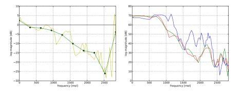
Gain function (yellow) and its parametrization (green). Source (blue), target (red), and warped and amplified source (green) magnitude spectra.
